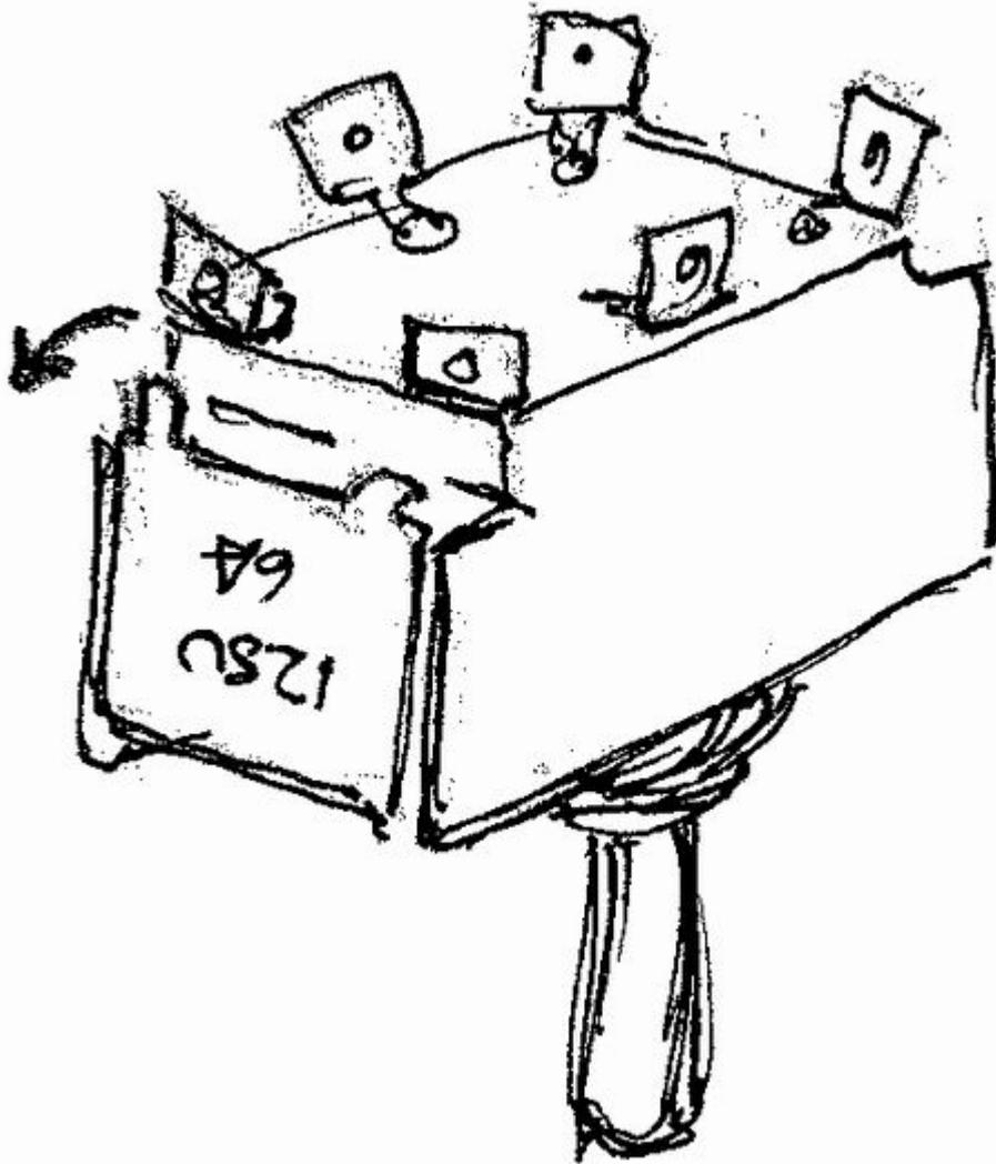
It **SHOULD** come apart like this. if your toggle switch doesn't have a rocking contact point as shown in the sketch, this DIY mod will not work.
