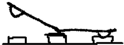
And place them like this. Each terminal should have one contact point touching on the opposite side of each other in the CENTER position of the toggle switch.
