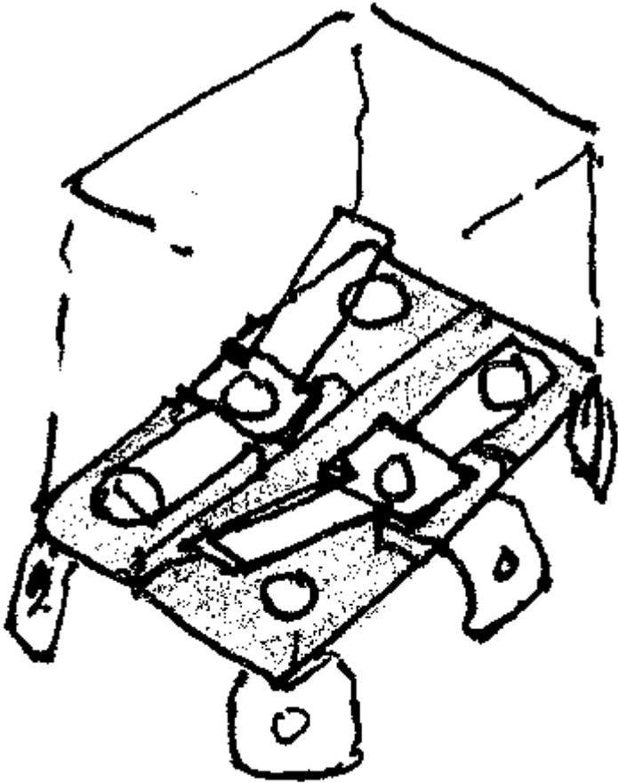
Then solder / connect the middle contact point. which goes to the output jack. You can either de-pin or leave the 3 unused terminals.
